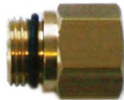
16 x 1.5 Male to 1/4 BSP Female Filling adaptor
